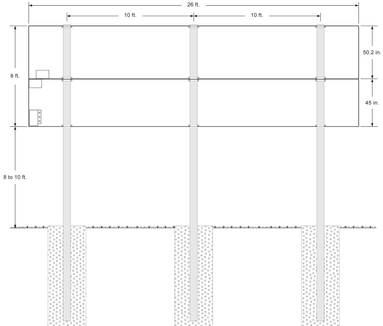
Once you have verified the positions of the posts and the size of the footings, you are ready to dig your holes, pour your concrete, and set your posts. There are several techniques for ensuring proper alignment of the posts. Typically installers will construct a temporary wooden support frame to hold each post in place while the concrete sets. Having plumb posts in the proper position is the key to a smooth mechanical installation.
