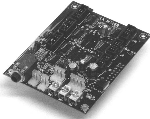
Data flows from one LX driver to the next in order, starting at the lower chassis (if there is more than one), and then left to right within each chassis. In the table(s) below, columns identify the LX Drivers, listed in order, left to right, based on the data path. The table rows give the names and purposes of the various connectors on the LX Drivers.
